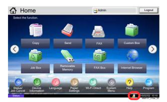
In Security Mode, the security kit has been properly installed and is running. The hard disk icon appears on the lower right side of the touch panel in Security Mode.
